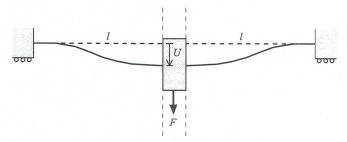
are clamped in blocks on their other ends (the latter are on rollers so as to provide unconstrained horizontal motion). All motions are without friction. What is the stiffness against a central force, i.e. F/U?
